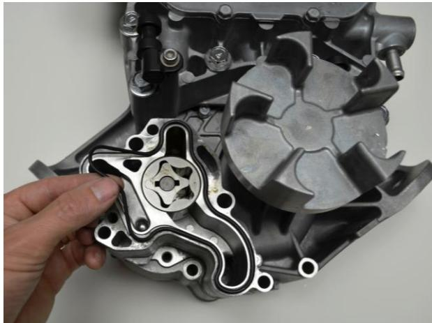
**Tip:** Apply grease to the new o-ring before installation. This will assist with holding the o-ring in place when reinstalling the oil pump cover.
